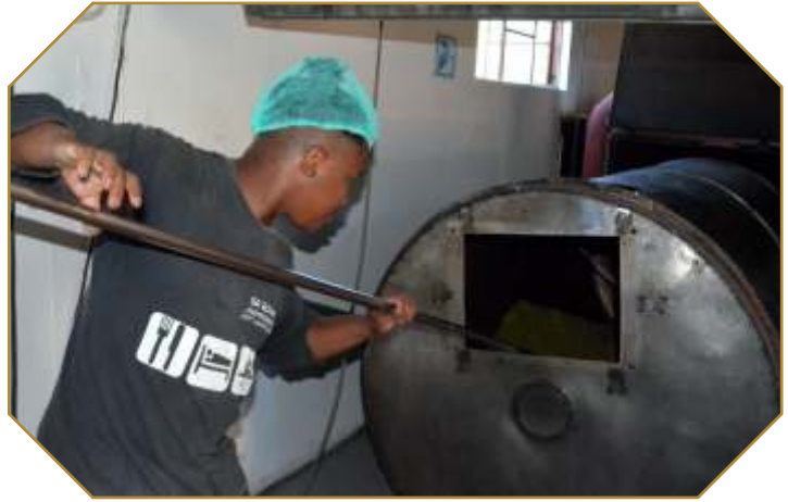
Fermenting the plant material: Quinzano Willeman is overlooking the process of heating up honeybush plant material in a stainless-steel drum for 70 hours at 70°C on the farm Nootgedacht. Photo by Heilie Combrink, courtesy of Netwerk24 .
